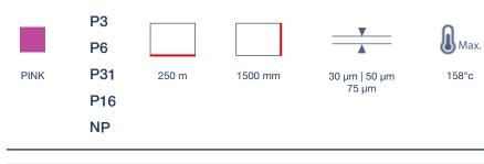
GFM-1R761-PK is a pink release film suitable for both resin infusion and prepreg processing. This product is compatible with all commonly used resin systems. In the non perforated version can work as self-releasing vacuum bagging film in debulking operations.
